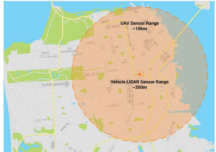
Figure 7 - RTK Can Aid in Extending Mapping Sensors Beyond the Autonomous Vehicle Local Sensor Suite
